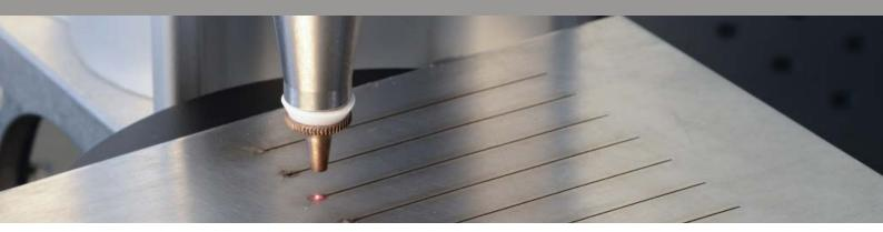
Integrated inline measurement system for an adaptive laser based cutting of complex surfaces
