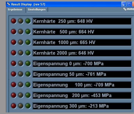
Result of a 3MA inspection
