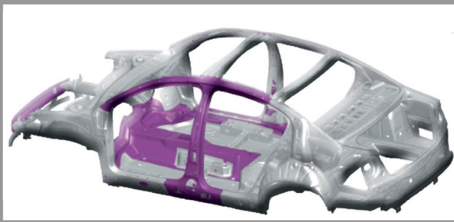
Reinforcing components of the car body Source: Volkswagen
