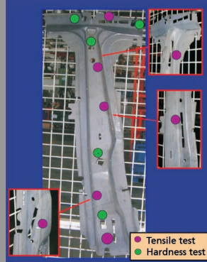
Component with flagged test positions ● Tensile test ● Hardness test
