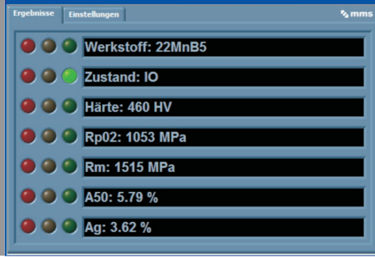
3MA result of press-hardened body part testing
