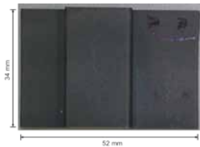
Component made of aluminum nitride: inhomogeneities detectable due to faulty nitration.
