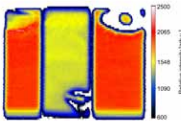
Component made of aluminum nitride: inhomogeneities detectable due to faulty nitration.
